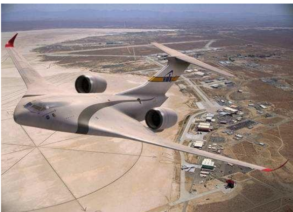
(a) Lockheed Martin's novel HBW configuration (Petrescu et al., 2018)
